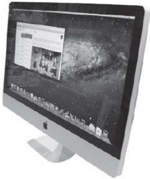
Figure 3.24 LED screens use a row of light-emitting diodes to backlight the display, resulting in better clarity, resolution, and color.
