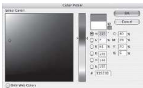
Figure 6.10 Color picker with HSB, RGB, and CMYK color models (Photoshop). See Color Plate 8.
