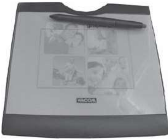
Figure 3.22 Artists and designers use graphics tablets and a stylus pen to input drawings for further editing.
