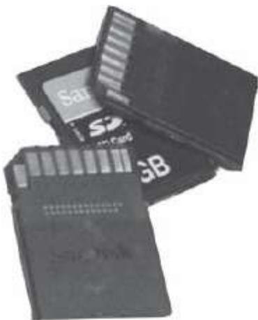
Figure 8.2 Digital video cameras are often equipped with solid-state storage media that offer light weight for ease of exchange and transport.
