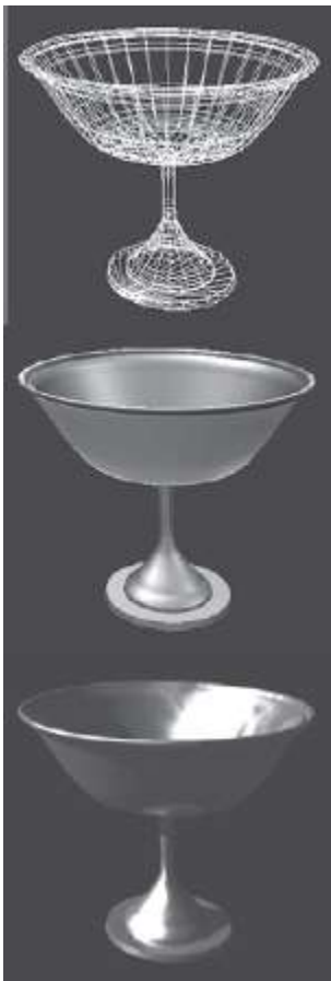
Figure 6.35 Rendering options: wire frame (top), smooth shading (middle) and ray tracing (bottom). See Color Plate 22.
